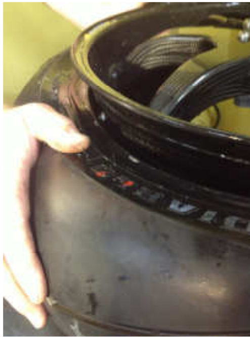
Figure 7: Keeping the tyre second tyre bead in the dip of the rim.
