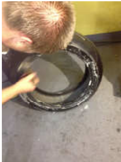
Figure 4: Applying soapy solution to the tyre walls.
