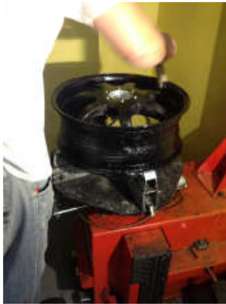
Figure 3: Applying soapy solution to the lip of the rim.
